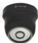
850 TVL Dome IR Camera 1/3" HDIS Sensor 850 TV Lines of Horizontal Resolution 0 Lux/F1.2 Min. Illumination (IR ON) 3.6 mm Fixed Lens 36 IR LED (10 Meters IR Range)
